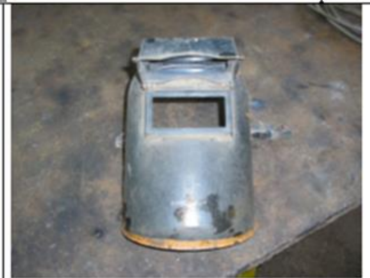
Welding helmet without safety glass – and we had many eye injuries this year.
